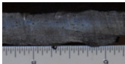
Figure 4 - Wrought iron plate showing internal imperfections
